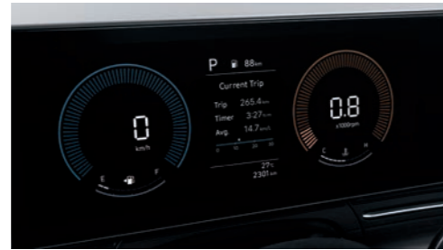
Cluster display (4-inch color LCD)* *Only available in Signature model
