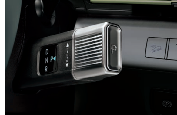
Column-Type Shift by Wire (SBW)* *Only available in Kona Hybrid model
