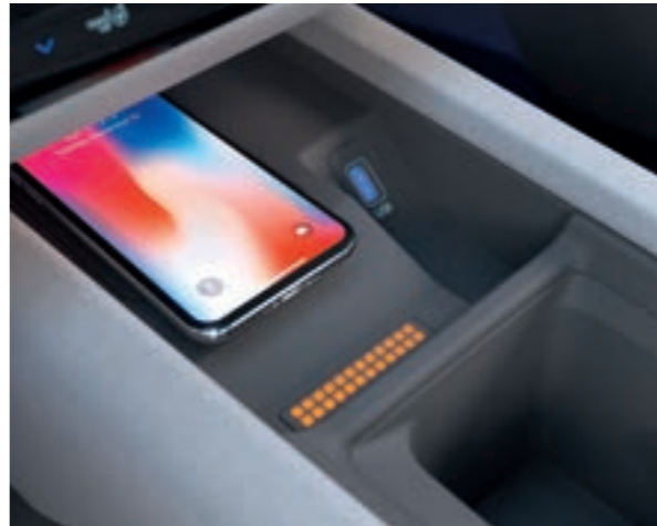
The high-speed wireless charger port features Parametric Pixels that signal the charge level of your smartphone at a glance.
